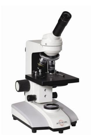
A tool that magnifies at a much higher power than a hand lens.
